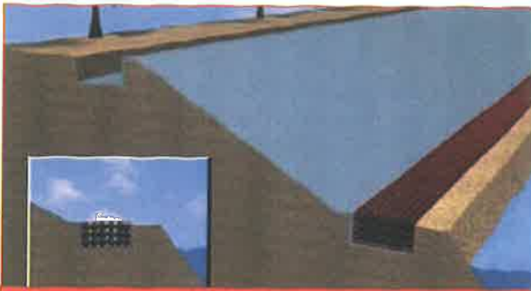
Metal Gabion Placed at Bottom Trench
