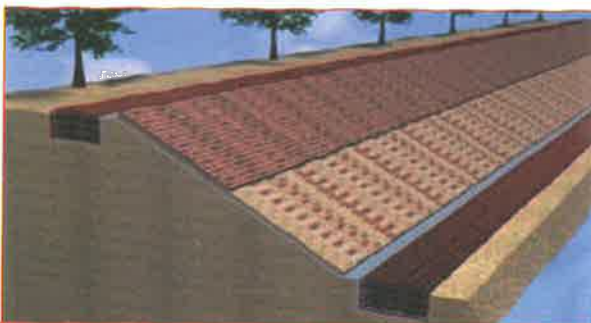
Two Layers of Brick Placed Along the Slope
