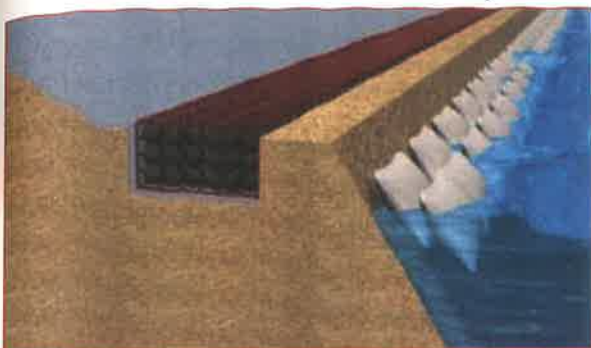
TechGeo Nonwoven Geotextile Bags in Two Layers at the Edge of the River Bed
