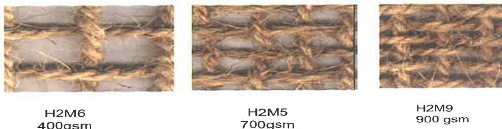
Fig.2. H_2M_6 , H_2M_5 , and H_2M_9 Netting of coir
