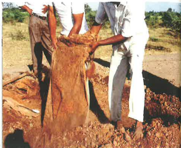
Geotextile excavated after 10 Years
