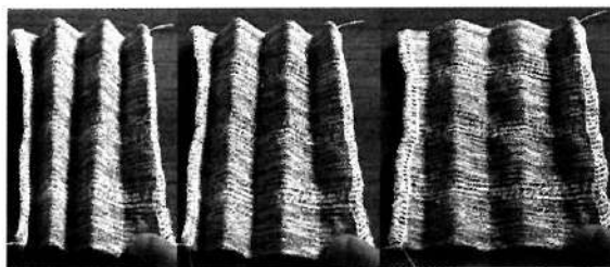
Figure 7. Shape Memory Recovery of SMP Composite Woven Uniformly and Densely of SMP Yarn at 50 °C with Recovery Time a) 0 s, b) 15 s, c) 30 s
