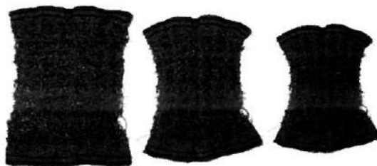
Figure 8. Shape Memory Recovery of SMP Composite Loosely Woven Fabric at 50 °C with recovery Time a) 0 s, b) 30 s, c) 60 s
